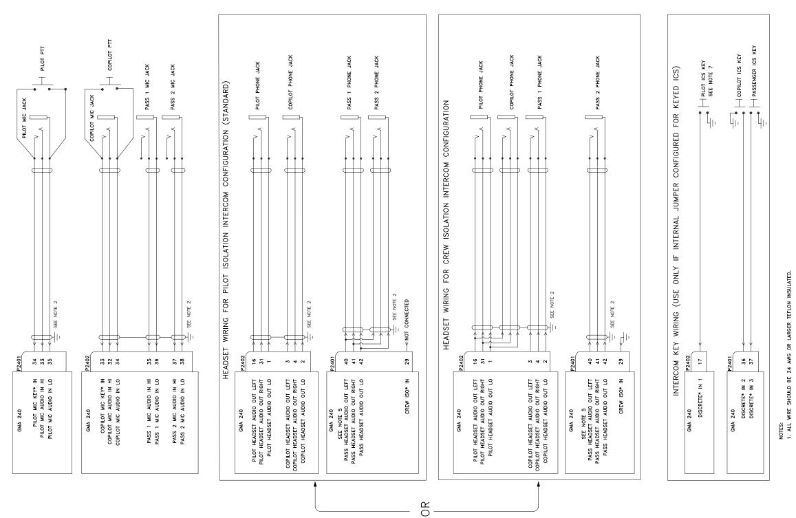
2. UNLESS OTHERWISE INDICATED, ALL SHIELDS MUST BE TERMINATED AT THE GMA 240 END ONLY. DAISY CHAIN SHIELDS A SUITABLE RING TERMINAL AND ATTACH TO CENTER GROUNDING LUGS IN BACK OF CONNECTOR BACKPLATE.
